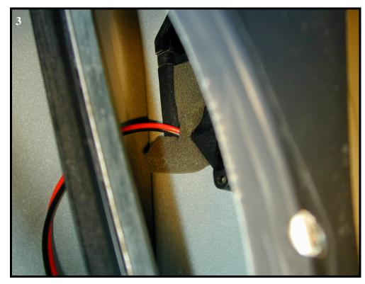
3. Guide the wire harnesses down into the door and bolt the mirror housing on the door. On the inside of the door there are two small holes at the bottom of where the plastic canister base is attached. The holes may be hidden behind foam insulation. Guide the wire harness through the left hole and out of the door.
